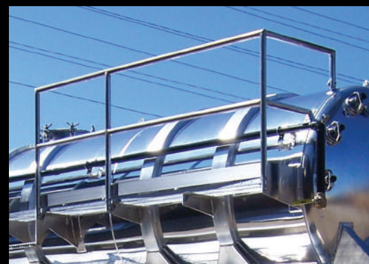
OSHA Catwalk and Guardrail
