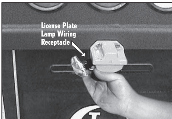
Figure 4.8 License Plate Lamp Replacement
