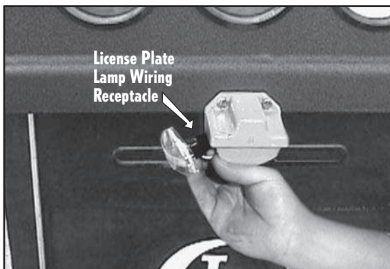
Figure 4.8 License Plate Lamp Replacement
